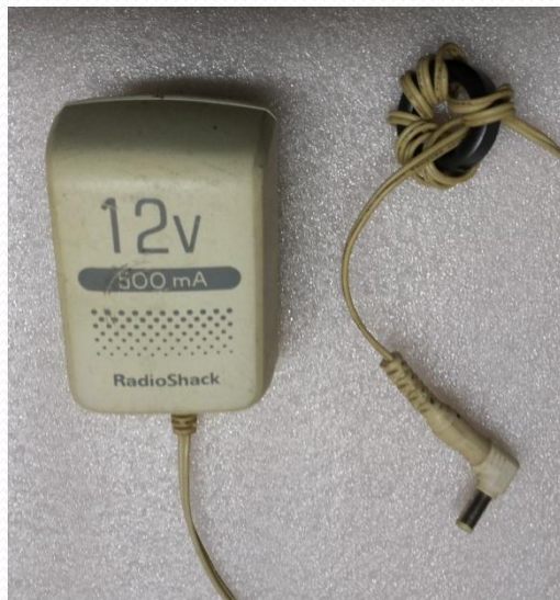
RFI Filter on DC Cord
