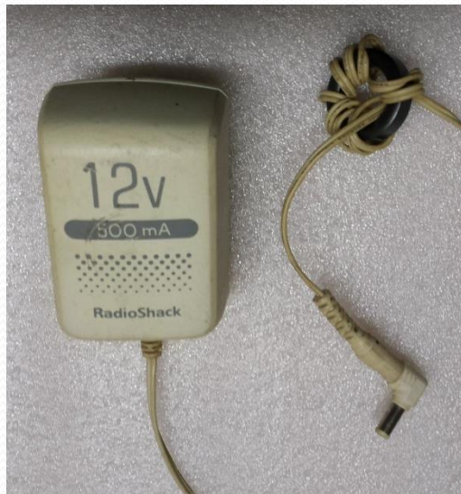
RFI Filter on DC Cord
