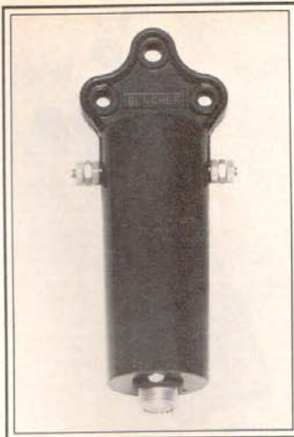
Bencher balun shown here is "pull tested" at 600 lbs. of antenna load, is rated at 5 kw peak power, and is fabricated of insulated, heavy-gauge, solid copper wire with an interwinding insulation of greater than 6000 volts. A ferrite core is not used in this design, which is said to be free of problems of saturation and loss at higher frequencies. Two models are available: the ZA-1, which is designed for 3.5-30 MHz operation, and the SA-2, which is optimized for 14-30 MHz and which includes stainless steel and aluminum hardware for a 2-inch boom. (Photo courtesy Bencher, Inc.)
