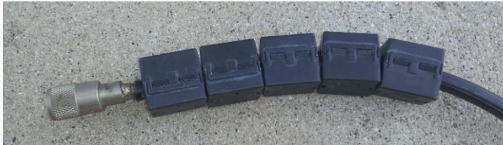
Snap On Choke 500-1000 \Omega 1-2 “S” Units
