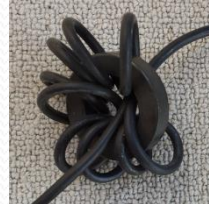
Ring Choke 1K-2K \Omega 2-4 “S” Units
