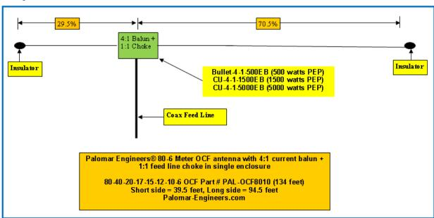
On the original antenna, the short side is 39.5 feet and on the new antenna with the RC-8040, the short side will be 38 feet. So adjust (DO NOT CUT WIRES) the length by pulling the excess 1.5 feet thru the insulator and wrapping it back on itself in case you have to make minor adjustment due to your overall antenna installation shape.
