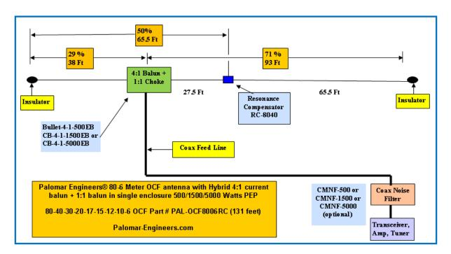
OCF antennas are very convenient as they will allow multiple bands of operation with a simple wire antenna which is fed off center.
