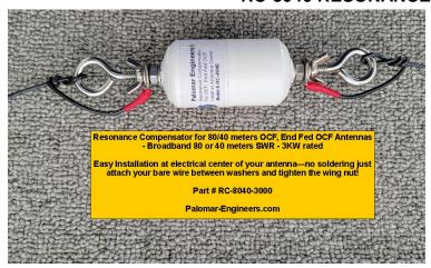
The resonance compensator is used to bring the 80 meter band resonance frequency closer to mid band as the natural length of the antenna must be cut for resonance in the lower portion of the 80 meter band so that 40, 20 and above band harmonics fall within their respective bands. The RC-8040 minimizes the amount of antenna tuner adjustment that may be required in the 80 meter band.
