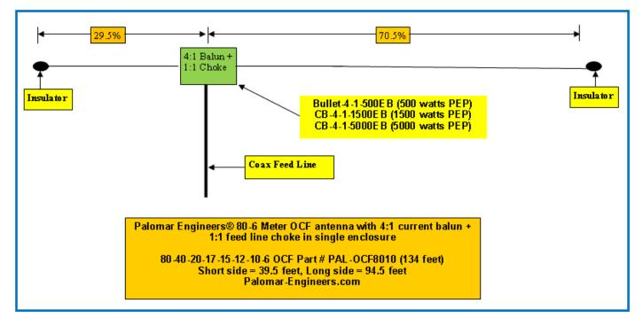
OCF antennas are very convenient as they will allow multiple bands of operation with a simple wire antenna which is fed off center. Rather than feeding the conventional 33%/67% we like the 29.5%/70.5% feed point wherein the feed point is 29.5% from one end and fed with a 4:1 OCF Current balun with built in 1:1 feed line choke the short side is 39.5 feet and the long side is 94.5 feet.
