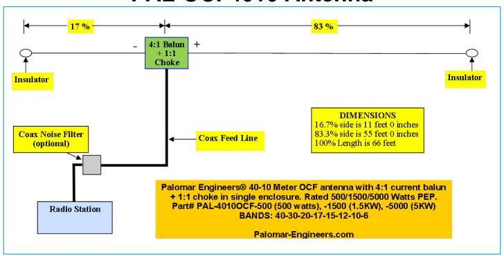
OCF antennas are very convenient as they will allow multiple bands of operation with a simple wire antenna which is fed off center. This antenna will work on 40-20-17-15-12-10 and 6 meters.
