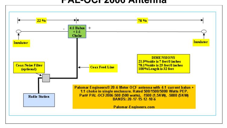
OCF antennas are very convenient as they will allow multiple bands of operation with a simple wire antenna which is fed off center. This antenna will work on 20-17-15-12-10 and 6 meters.
