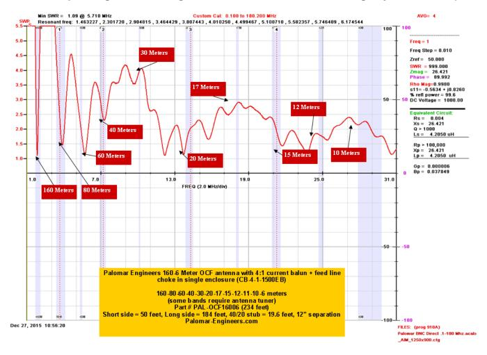
Note: Second stub (under the longest part of OCF) has the effect of shortening the overall antenna length to 234 feet. If you do not want the second stub, then make the antenna 260 feet long with legs of 79% and 21% of the total length.
