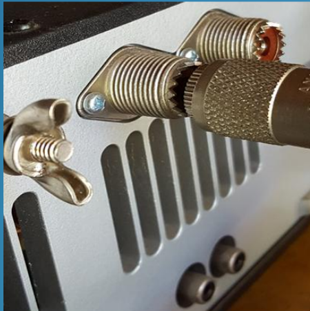
Coax Center Conductor Only—measure noise level
