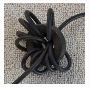
Coax Noise Filter .1-150 MHz >2K 500 Watts PEP 1K-6K Z -  $50\Omega$ 1/2 pound, rugged
