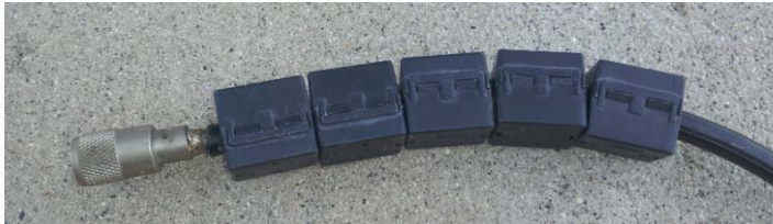
Snap On Choke 500-1000 \Omega
