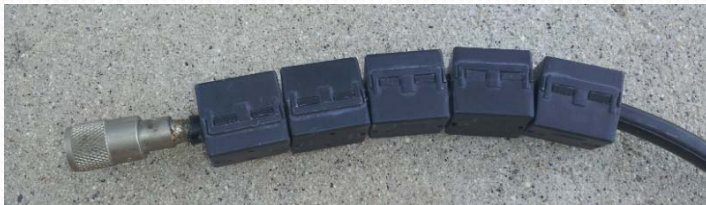
Snap On Choke 500-1000 \Omega - Good
