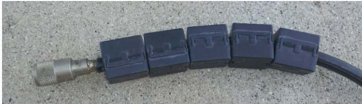
Snap On Choke 500-1000 \Omega
