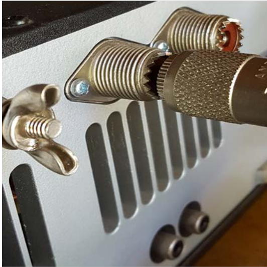
Coax Center Conductor Only—measure noise level
