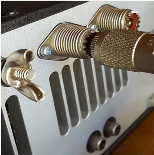
Coax Center Conductor Only—measure noise level
