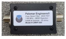
If the distance from the coax feed line choke is over 25 feet, it may be beneficial to use a coax noise filter which <u>suppresses common mode noise picked up on the coax outer braid during RECEIVE operation</u>. You hear this "noise" as a higher than normal noise floor when you connect the outside of the coax connector to your radio. Vertical antennas in general have a higher noise factor due to the vertical polarity nature of noise sources in the neighborhood.
