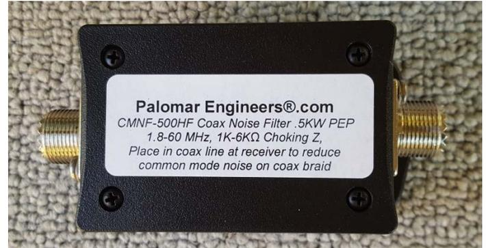
To install, simply connect the coax line from the antenna to one connector and add a small coax jumper from the other connector to your radio. This encapsulated filter is also more durable than the ferrite ring which can fracture if dropped on the ground.
