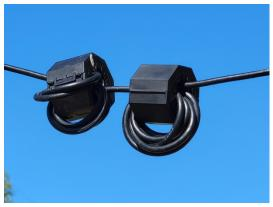
If you use RG-8X size cable, then the included SOFLCx2 with this kit is sufficient if you have 5-6 turns thru the center of each. See picture on next page as an example of how to wind the cable.
