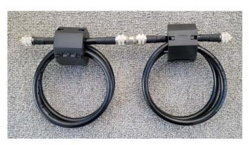
If you use LMR-400 or 1/2" coax cable you will only get 3 turns thru the snap on choke and you will need an additional choke (with an additional 3 turns) in series to provide enough choking on 40 and 80 meters. Part# SOFLC.
