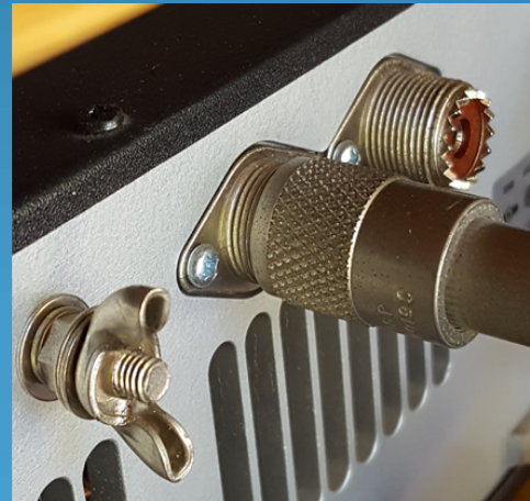
Coax Center Conductor and outer shield — measure noise level. If higher, then you have common mode noise
