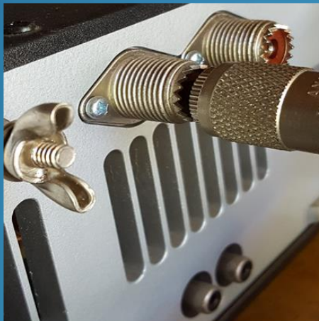
Coax Center Conductor Only—measure noise level
