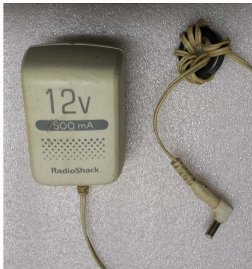
RFI Filter on DC Cord
