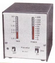
M-827 SPECIFICATIONS: Frequency Range: 1-30 MHz. SWR Display: 1.0 to 10 SWR. Logarithmic expanded scale. Power Ranges: 0-20, 0-200, 0-2000 watts selected by panel switch. Controls: On-off, power range. Connectors: Input and Output UHF type S0-239. Power Required: 115v 50/60 Hz. Size:  $10\times10\times13$  cm ( $4\times4\times5$  in. deep). Weight: 800-g ( $1^4$ -lb.) Cabinet: Brushed aluminum panel, black vinyl cover.
